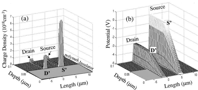
FIG. 3. Calculated 2D distribution of the hole density (a) and the electrostatic potential (b) 150n after the gate bias was set to  $-5\text{ V}$  ( $V_S=0$ ,  $V_D=-3\text{ V}$ ).
