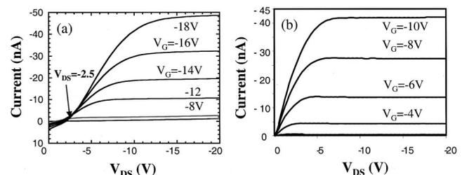
FIG. 2. Measured drain current for TOC (a) and BOC (b) structures. The channel lengths were 40 μm and 10 μm respectively.
