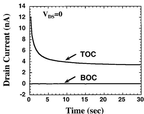
FIG. 5. Measured drain current as a function of time after applying a gate bias. TOC curve was measured in the TOC structure and the BOC curve for the BOC one.
