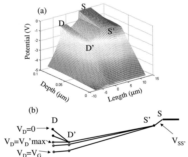
FIG. 4. (a) Calculated 2D potential distribution for the TOC structure. The transistor active region has reached its steady state. (b) Schematic description of the potential distribution between the contacts for varying drain voltage.
