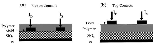
FIG. 1. Schematic description of TOC and BOC FET structures.
