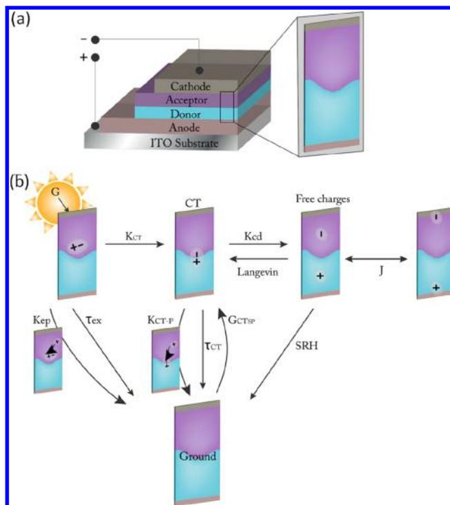
**Figure 2.** (a) 3D device structure and illustration of a process block to be used in (b). (b) Flow diagram of the processes accounted for in the basic model used here.
