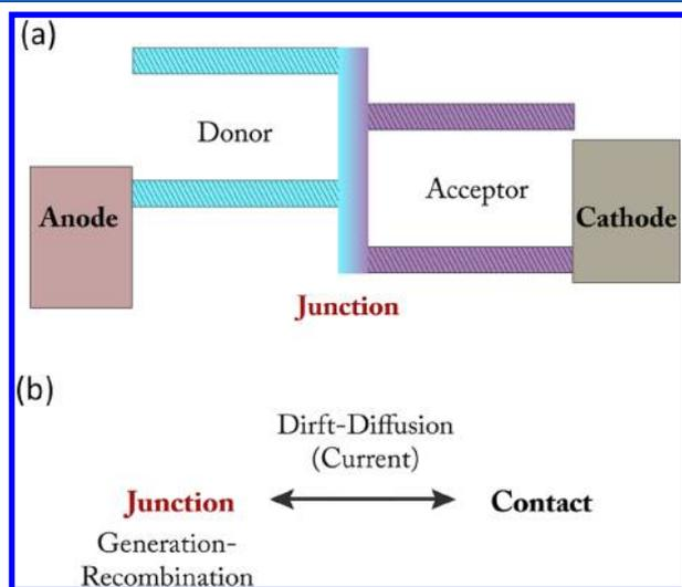
**Figure 1.** (a) Schematic description of a planar heterojunction organic photocell. (b) Illustration of the modeling concept used here.
