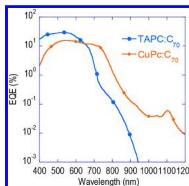
**Figure 4.** EQE as a function of excitation wavelength for CuPc:C<sub>70</sub>- and TAPC:C<sub>70</sub>-based devices.
