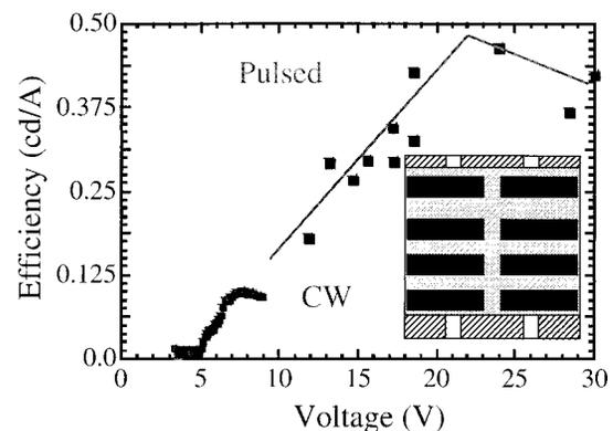
FIG. 1. Device efficiency as a function of applied voltage. The bottom line was measured under cw conditions and the square markers under short pulse, low duty cycle, conditions. The line is a guide to the eye. The inset shows the LED configuration from bottom up: ITO, Al covered by Al<sub>2</sub>O<sub>3</sub>, polymer layers, contact layers.
