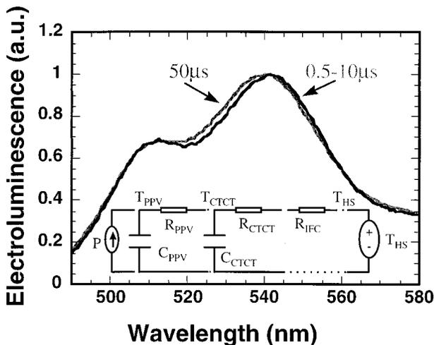
FIG. 3. Average emission spectra taken with pulses of differing duration. The inset shows the device equivalent circuit.
