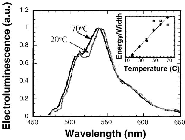
FIG. 2. Average emission spectra measured at two heat-sink temperatures (20 and 70 °C). The inset shows the change of peak energy and width as a function of temperature.
